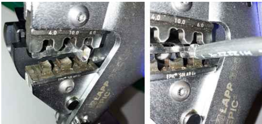
Contact in the crimp insert
