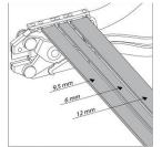
4. Push the holder through the hole for punching the following holes for cable tie mounting
