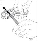
5. Use the front cutting part to cut the punched holders
