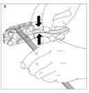
6. Use the front punching part for punching center holes for screw mounting
